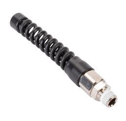
NITRA pneumatic or water threaded fitting, male, hose rigid, nickel-plated brass body, nickel-plated brass threads, thread sealant, 1/4in inside diameter to 1/4in male NPT.
