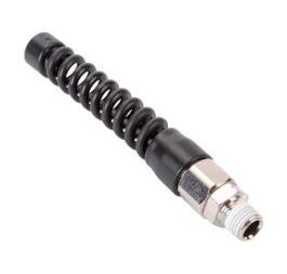
NITRA air or water threaded fitting, male, hose rigid, nickel-plated brass body, nickel-plated brass threads, thread sealant, 1/4in inside diameter to 1/4in male NPT.
