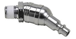
NITRA pneumatic quick disconnect fitting, swivel, chrome-plated steel body, (1) 1/4in male NPT to (1) 1/4in industrial interchange.
