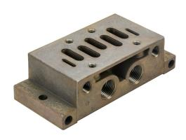
NITRA air stand-alone base, aluminum alloy, 145 psi (10 bar) maximum operating pressure, 3/8in female NPT inlet(s), 3/8in female NPT outlet(s), 3/8in female NPT exhaust(s), side orientation. For use with ISO 5599/1 size 2 solenoid valves.
