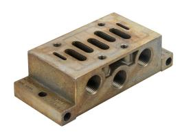
NITRA air stand-alone base, aluminum alloy, 145 psi (10 bar) maximum operating pressure, G3/8 female BSPP inlet(s), G3/8 female BSPP outlet(s), G3/8 female BSPP exhaust(s), side orientation. For use with ISO 5599/1 size 2 solenoid valves.
