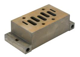
NITRA air stand-alone base, aluminum alloy, 145 psi (10 bar) maximum operating pressure, G3/8 female BSPP inlet(s), G3/8 female BSPP outlet(s), G3/8 female BSPP exhaust(s), bottom orientation. For use with ISO 5599/1 size 2 solenoid valves.
