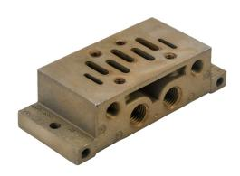
NITRA air stand-alone base, aluminum alloy, 145 psi (10 bar) maximum operating pressure, 1/4in female NPT inlet(s), 1/4in female NPT outlet(s), 1/4in female NPT exhaust(s), side orientation. For use with ISO 5599/1 size 1 solenoid valves.
