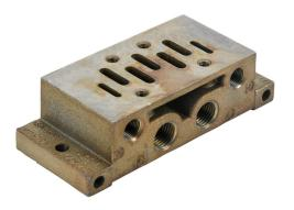
NITRA air stand-alone base, aluminum alloy, 145 psi (10 bar) maximum operating pressure, G1/4 female BSPP inlet(s), G1/4 female BSPP outlet(s), G1/4 female BSPP exhaust(s), side orientation. For use with ISO 5599/1 size 1 solenoid valves.
