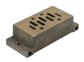
NITRA air stand-alone base, aluminum alloy, 145 psi (10 bar) maximum operating pressure, 1/4in female NPT inlet(s), 1/4in female NPT outlet(s), 1/4in female NPT exhaust(s), bottom orientation. For use with ISO 5599/1 size 1 solenoid valves.
