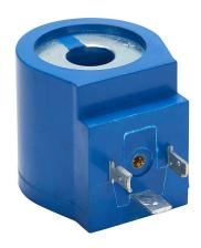
GC Valves solenoid coil, replacement, 24 VDC, 10W, 18mm DIN style wiring plug. For use with S201, NS201, S211 DC, NS211 DC, S301 and NS301 valves.
