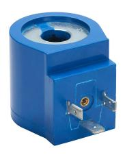
GC Valves solenoid coil, 240 VAC, 10W, 18mm DIN style wiring plug. For use with S201, NS201, S301 and NS301 valves.
