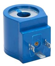
GC Valves solenoid coil, replacement, 120 VAC, 10W, 18mm DIN style wiring plug. For use with S201, NS201, S301 and NS301 valves.
