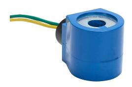
GC Valves solenoid coil, 24 VDC, 10W, 24in 18AWG pigtail. For use with S201, NS201, S211 DC, NS211 DC, S301 and NS301 valves.
