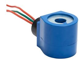
GC Valves solenoid coil, 240 VAC, 10W, 24in 18AWG pigtail. For use with S201, NS201, S301 and NS301 valves.
