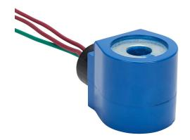
GC Valves solenoid coil, 120 VAC, 10W, 24in 18AWG pigtail. For use with S201, NS201, S301 and NS301 valves.
