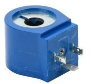
GC Valves solenoid coil, replacement, 24 VDC, 9W, 18mm DIN style wiring plug. For use with S211 series valves.
