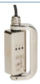
IDEM Z-Range safety switch, right hand door hinge interlock, (2) OSSD safety output(s), (1) status monitoring output(s), 316 stainless steel housing, 120 x 66mm, pigtail, 16.4ft/5m cable length.
