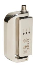
IDEM Z-Range safety switch, left hand door hinge interlock, (2) OSSD safety output(s), (1) status monitoring output(s), 316 stainless steel housing, 120 x 66mm, 8-pin M12 quick-disconnect, 9.8in/250mm cable length.
