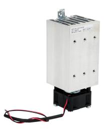
Gefran heatsink with fan, 35mm DIN rail mount. For use with Gefran GQ series solid state relays up to 75A. Mounting hardware included.
