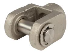
NITRA cylinder rod clevis, M22 x 1.5 thread, cast iron. For use with 80mm H-series cylinders. Male adapter and hex nut included.
