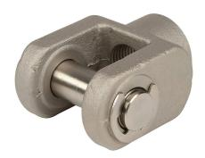
NITRA cylinder rod clevis, M18 x 1.5 thread, cast iron. For use with 63mm H-series cylinders. Male adapter and hex nut included.
