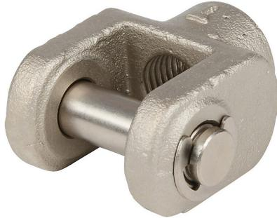
NITRA cylinder rod clevis, M14 x 1.5 thread, cast iron. For use with 32mm H-series cylinders. Male adapter and hex nut included.
