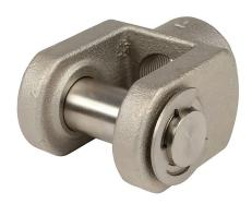
NITRA cylinder rod clevis, M26 x 1.5 thread, cast iron. For use with 100mm H-series cylinders. Male adapter and hex nut included.
