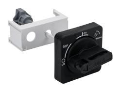
IronHorse rotary handle, selector, black, external front mount, 2-position, lockable in ON-OFF, defeatable, NEMA 3R, IP65. For use with HMMP-100H manual motor protectors. 115mm shaft, operator and mounting screws included.
