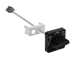
IronHorse rotary handle, selector, black, external front mount, 2-position, lockable in ON-OFF, defeatable, NEMA 3R, IP65. For use with HMMP-63H manual motor protectors. 315mm shaft, operator and mounting screws included.
