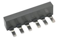
IronHorse busbar, 108A, 600 VAC, cut to length not permitted, connects up to 2 HMMP-63H Manual motor protectors without accessories.
