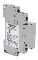
IronHorse field installable alarm contact, left side mount, (1) N.O./ (1) N.C. contact(s), 6A @ 120 VAC/0.55A @ 120 VDC, screw terminal. For use with HMMP-63H and HMMP-100H manual motor protectors.
