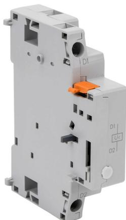
IronHorse field installable undervoltage trip, right side mount, 460-480 VAC (60Hz)/415-440 VAC (50Hz) sensing range, screw terminal. For use with HMMP-32H to HMMP-100H manual motor protectors.
