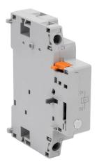
IronHorse field installable undervoltage trip, right side mount, 460-480 VAC (60Hz)/415-440 VAC (50Hz) sensing range, screw terminal. For use with HMMP-32H to HMMP-100H manual motor protectors.
