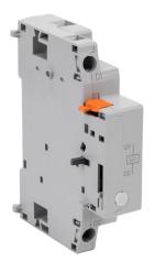
IronHorse field installable undervoltage trip, right side mount, 200-220 VAC (60Hz)/200 VAC (50Hz) sensing range, screw terminal. For use with HMMP-32H to HMMP-100H manual motor protectors.
