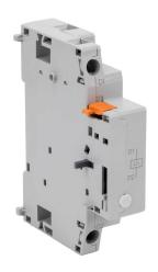
IronHorse field installable undervoltage trip, right side mount, 120 VAC (60Hz)/110 VAC (50Hz) sensing range, screw terminal. For use with HMMP-32H to HMMP-100H manual motor protectors.
