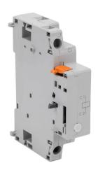
IronHorse field installable shunt trip, right side mount, 460-480 VAC (60Hz)/415-440 VAC (50Hz) coil voltage, screw terminal. For use with HMMP-32H to HMMP-100H manual motor protectors.
