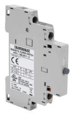
IronHorse field installable short circuit alarm contact, left side mount, (1) N.O./(1) N.C. contact(s), 6A @ 120 VAC/0.55A @ 120 VDC, screw terminal. For use with HMMP-32H to HMMP-100H manual motor protectors.
