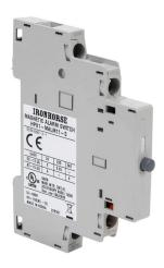
IronHorse field installable short circuit alarm contact, left side mount, (1) N.O./(1) N.C. contact(s), 6A @ 120 VAC/0.55A @ 120 VDC, screw terminal. For use with HMMP-32H to HMMP-100H manual motor protectors.
