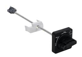
IronHorse rotary handle, selector, black, external front mount, 2-position, lockable in ON-OFF, defeatable, NEMA 3R, IP65. For use with HMMP-32H manual motor protectors. 315mm shaft, operator and mounting screws included.
