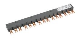
IronHorse busbar, 64A, 600 VAC, cut to length not permitted, connects up to 5 HMMP-32H Manual motor protectors without accessories. Use HPX1-PTB-MP power terminal to connect feeder.
