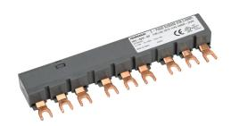
IronHorse busbar, 64A, 600 VAC, cut to length not permitted, connects up to 3 HMMP-32H Manual motor protectors without accessories. Use HPX1-PTB-MP power terminal to connect feeder.
