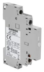
IronHorse field installable auxiliary contact, left side mount, (2) N.O. contact(s), 6A @ 120 VAC/0.55A @ 120 VDC, screw terminal. For use with HMMP-32H to HMMP-100H manual motor protectors.
