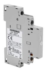
IronHorse field installable auxiliary contact, left side mount, (1) N.O./(1) N.C. contact(s), 6A @ 120 VAC/0.55A @ 120 VDC, screw terminal. For use with HMMP-32H to HMMP-100H manual motor protectors.
