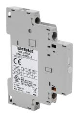
IronHorse field installable auxiliary contact, left side mount, (2) N.C. contact(s), 6A @ 120 VAC/0.55A @ 120 VDC, screw terminal. For use with HMMP-32H to HMMP-100H manual motor protectors.
