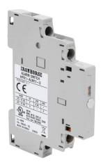
IronHorse field installable alarm contact, left side mount, (1) N.O./ (1) N.C. contact(s), 6A @ 120 VAC/0.55A @ 120 VDC, screw terminal. For use with HMMP-32H manual motor manual motor protectors.
