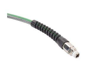
NITRA pneumatic or water hose, hybrid PVC, polyester reinforced, black with green stripe, 1/4in inside diameter, 7/16in outside diameter, 1/4in male NPT nickel-plated brass rigid fittings, 50ft.
