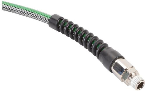
NITRA pneumatic or water hose, hybrid PVC, polyester reinforced, black with green stripe, 1/4in inside diameter, 7/16in outside diameter, 1/4in male NPT nickel-plated brass rigid fittings, 50ft.
