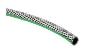
NITRA pneumatic or water hose, hybrid PVC, polyester reinforced, black with green stripe, 1/4in inside diameter, 7/16in outside diameter, 500ft.
