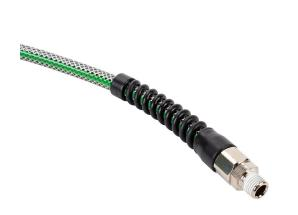
NITRA pneumatic or water hose, hybrid PVC, polyester reinforced, black with green stripe, 1/4in inside diameter, 7/16in outside diameter, 1/4in male NPT nickel-plated brass rigid fittings, 25ft.
