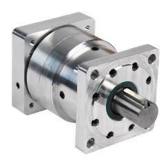
SureGear high-precision strain wave gearbox, 80:1 ratio, inline, 1in diameter output shaft, nominal output torque 40 N-m (354 lb-in), 1-stage, NEMA 34 frame. For use with SureStep NEMA 34 motors.
