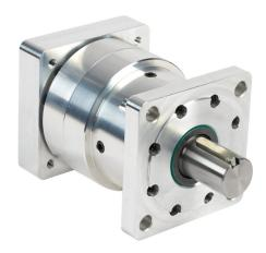
SureGear high-precision strain wave gearbox, 50:1 ratio, inline, 1in diameter output shaft, nominal output torque 40 N-m (354 lb-in), 1-stage, NEMA 34 frame. For use with SureStep NEMA 34 motors.
