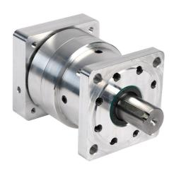
SureGear high-precision strain wave gearbox, 120:1 ratio, inline, 1in diameter output shaft, nominal output torque 50 N-m (443 lb-in), 1-stage, NEMA 34 frame. For use with SureStep NEMA 34 motors.
