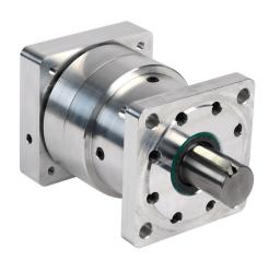
SureGear high-precision strain wave gearbox, 100:1 ratio, inline, 1in diameter output shaft, nominal output torque 50 N-m (443 lb-in), 1-stage, NEMA 34 frame. For use with SureStep NEMA 34 motors.
