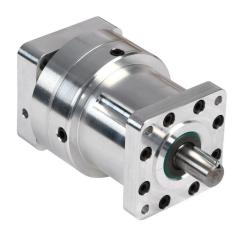
SureGear high-precision strain wave gearbox, 100:1 ratio, inline, 0.5in diameter output shaft, nominal output torque 30 N-m (266 lb-in), 1-stage, NEMA 23 frame. For use with SureStep NEMA 23 motors.
