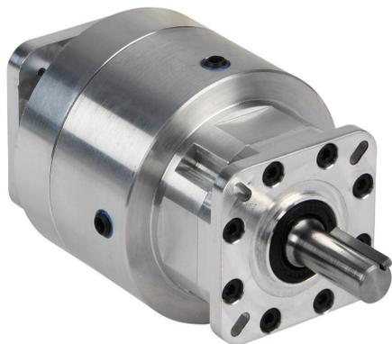
SureGear high-precision strain wave gearbox, 80:1 ratio, inline, 0.375in diameter output shaft, nominal output torque 12 N-m (106 lb-in), 1-stage, NEMA 17 frame. For use with SureStep NEMA 17 motors.
