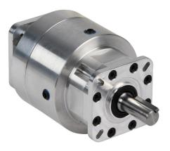
SureGear high-precision strain wave gearbox, 80:1 ratio, inline, 0.375in diameter output shaft, nominal output torque 12 N-m (106 lb-in), 1-stage, NEMA 17 frame. For use with SureStep NEMA 17 motors.
