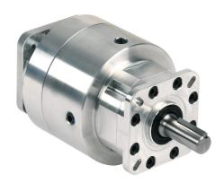
SureGear high-precision strain wave gearbox, 50:1 ratio, inline, 0.375in diameter output shaft, nominal output torque 12 N-m (106 lb-in), 1-stage, NEMA 17 frame. For use with SureStep NEMA 17 motors.
