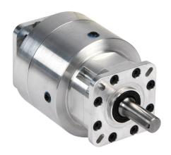
SureGear high-precision strain wave gearbox, 100:1 ratio, inline, 0.375in diameter output shaft, nominal output torque 15 N-m (133 lb-in), 1-stage, NEMA 17 frame. For use with SureStep NEMA 17 motors.
