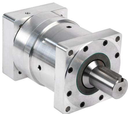
SureGear high-precision strain wave gearbox, 80:1 ratio, inline, 32mm diameter output shaft, nominal output torque 100 N-m (885 lb-in), 1-stage, 116mm frame. For use with SureServo and SureServo2 SV(2)L-210(B) motors.
